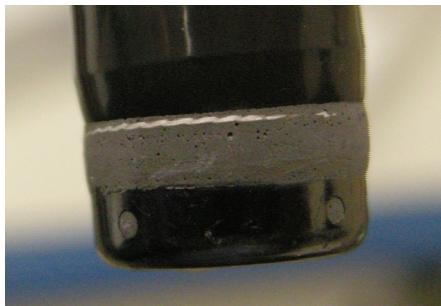
Deterioration and pitting of adhesive at bending section and insertion tube junction
