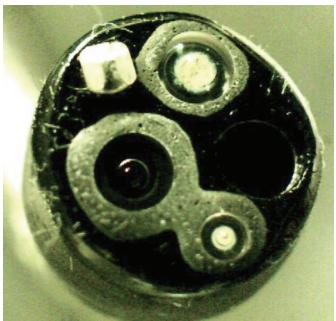
Deterioration and pitting of adhesive at bending section and distal end junction
