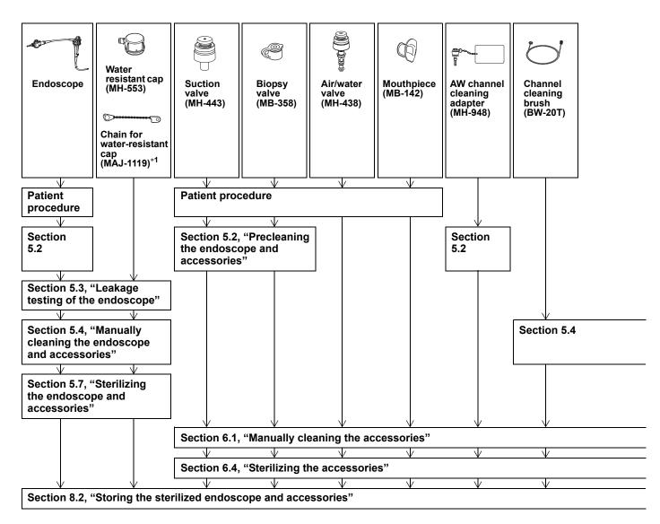
\*1 The water resistant cap (MH-553) should remain connected to the endoscope at all times using the chain for water-resistant cap (MAJ-1119).
