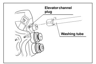
1. Attach the washing tube to the elevator channel plug.
